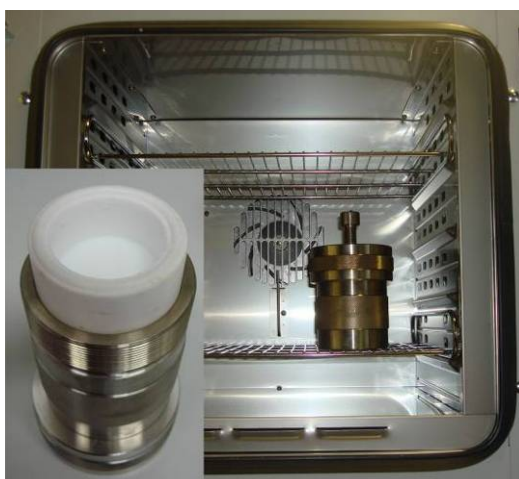
Figure 26: Autoclave . Metallic autoclave (on the inset) with inner Teflon cartridge in the furnace.
