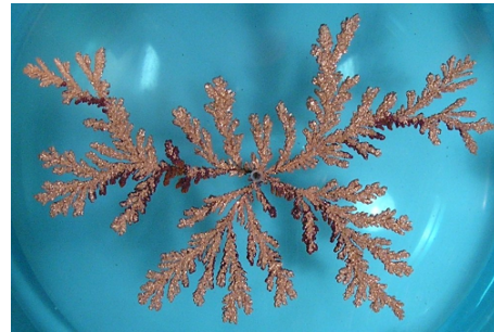
Figure 17: A DLA cluster grown from a copper (II) sulphate solution in an electrodeposition cell [6]. Fractals are tree-like. The shapes depend on the applied voltage and the concentration of electrolyte. A linear geometry can also be adopted with growth between parallel electrodes.
