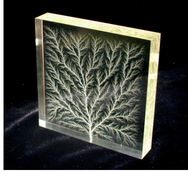
Figure 18: High-voltage dielectric breakdown (HVDB) within a block of plexiglas creates a fractal pattern [6]. Dielectric breakdown refers to the formation of electrically conducting regions in an insulating material exposed to a strong electric field. HVDB represents the negative of DLA when fractal grows from particles from the environment.
